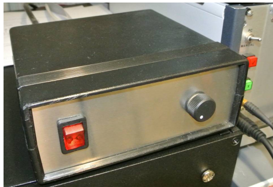
Figure 5: The illuminator power supply.
